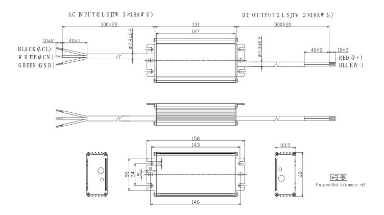
**Safety Note:** Please make sure the output cable does not connect to dimming cable or the cables of other drivers until 20 seconds after being tested because of the remained voltage in the output capacitor.
